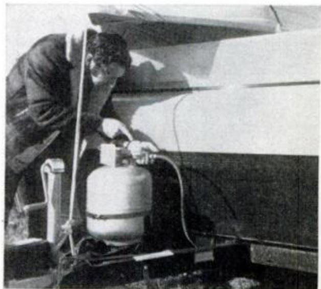
USE ONLY PROPANE GAS or a propane blend for winter camping. Butane will not vaporize below 32°F. Also, insulate your gas regulator in some way
